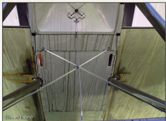
Fuselage detail from E8102 showing aluminium undershield panels (usually painted service grey), elevator control horn clearance slots and, once again, extensive caster oil staining.
