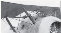
Center section and strut detail from an unidentified late production Sopwith Snipe. Note the painted center section struts, fuel system venturi (A8), Brackets For Aldis sight (A34) (without the Aldis sight (A33)), windscreen (C) and ring & bead sight (P2 & P4). The Vickers Mk.1* cooling jackets appear to have also been painted grey.
