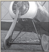
Undercarriage detail from an unidentified late production Sopwith Snipe. Note the dark suspension bungee cord and how subtle the traditional Sopwith split axle angle is on the Snipe compared to earlier designs like the Triplane and Pup (see Wingnut Wings models 32008, 32013 and 32016). Almost all Sopwith Snipe propellers had their blades wrapped in linen and painted grey and display no manufacturer decals, although we have included optional Lang decals [88] for you to use if you wish.
