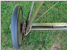
Undercarriage detail from E8102 showing the split axle, bungee suspension cord and extensive caster oil staining.
